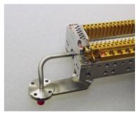
Figure 1: Magic fingers at the four magnet girder ends. Each slot is filled with a transversally quadratic permanent magnet of a specific thickness.
