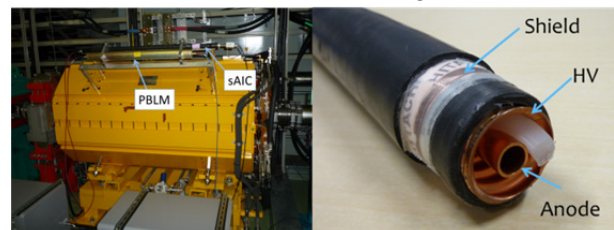
Figure 1: Left) Photo of the PBLM and sAIC. Right) Cable structure used for AIC.
