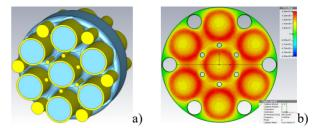
Figure 4: MBK bunching cavity design (a) where drift tubes and rods are given in yellow and vacuum volume in blue. Contour plot of the field distribution in median plane (b). The outer dimension is  $\emptyset$ 34 mm (1.3").
