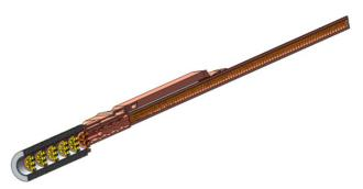
Figure 10: Rendering of the  $\emptyset$ 3.5" KlyLac design with MBK and 2-port linac section (see Fig. 7). MBK cathode and linac focusing are not shown.
