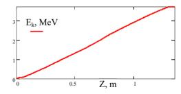
Figure 13: Beam energy gain [MeV] along the structure for the field profile of Fig. 8 (bottom) for RF power ~600 kW.
