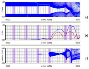
Figure 2: AJDisk simulations for a single beamlet of sixcavity, 7-beam X-band MBK for KlyLac with phase (a), bunching factors for fundamental and next harmonic (b), and particle velocities plotted along the klystron.
