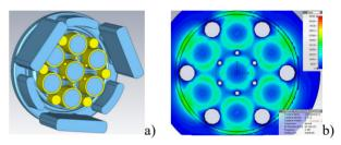
Figure 5: Upstream view (a) of the output MBK cavity. Contour plot of the field distribution in median plane (b).
