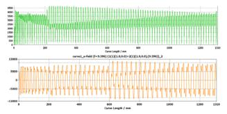
Figure 8: Ez field profiles along the 3-port (magnitude on the top) and 2-port (bottom) configurations of Fig. 6.
