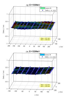
Figure 3: Beam offset in x-plane (bottom) and in y-plane (top) as a function of the scanned beam deflection.
