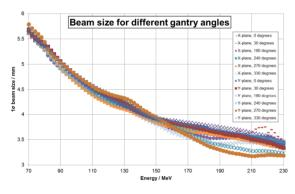
Figure 2: Beam size at the iso-center as a function of energy for different gantry angle settings.
