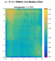
Figure 4: Dose distribution for a full scan field with an applied mono-energetic layer of 90 MeV. The color-wash scale is indicated on the right hand side of the figure.
