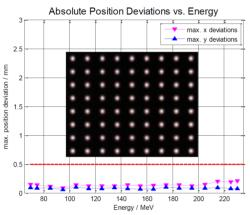
Figure 5: Absolute deviation of beam position in x and y as a function of beam energy and an example of measured distribution of the scanned beam.
