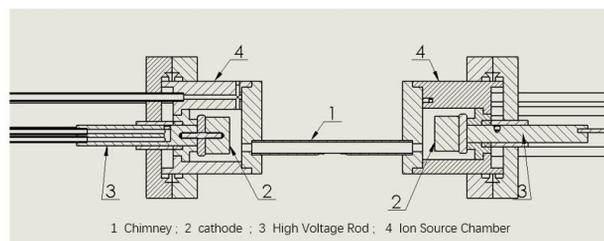
Figure 1: Structure of the PIG source.
