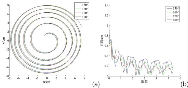
Figure 7: Beam orbit with different initial phase; (a)Particle orbits; (b)Particle orbit curvature center.
