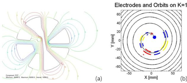
Figure 6: (a):Electric field of the central region;(b)Typical beam orbit.
