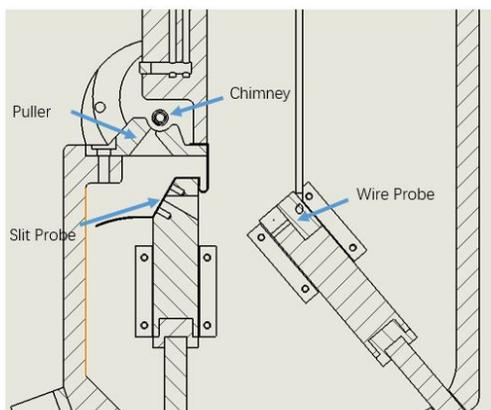
Figure 4: Structure of the ion source testing chamber.
