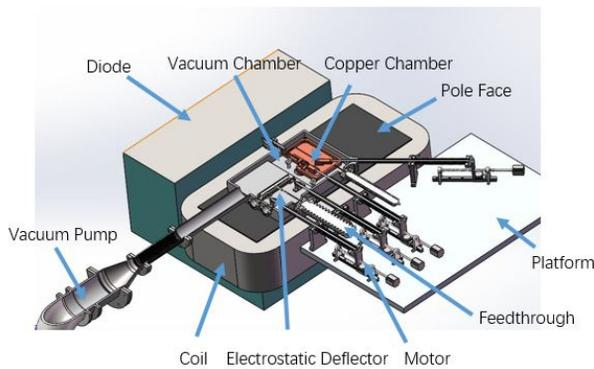
Figure 3: Structure of the ion source test bench.
