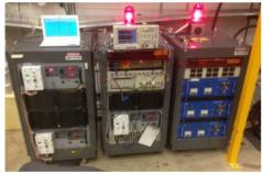
Figure 7: Charging pulser tower (left), the control tower (center) and the thyratrons PS tower (right).
