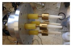
Figure 4: End of transmission line. Conical fingers serve for capturing theirs own resistor from Fig. 3 during insertion.
