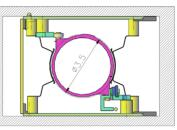
Figure 5: E-989 kicker cross-section. The NMR cartridge profile in measuring position is shown also. Diameter of circle is  $\sim$ 89 mm (3.5").
