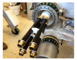
Figure 3: The Kicker input. Four load resistors are Kanthal tubular resistors,  $50\Omega$  each. Cylindrical protective cover removed. Inner volume is filled with Fluorinert FC-40.
