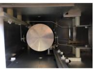
Figure 6: NMR cartridge is running on the rails between the kicker plates. Input jumper is visible at the top.
