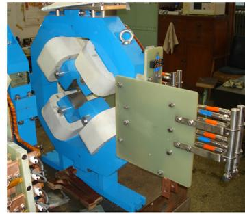
Figure 3: NSC KIP 100 MeV/100 kW linear accelerator quadrupole lens.
