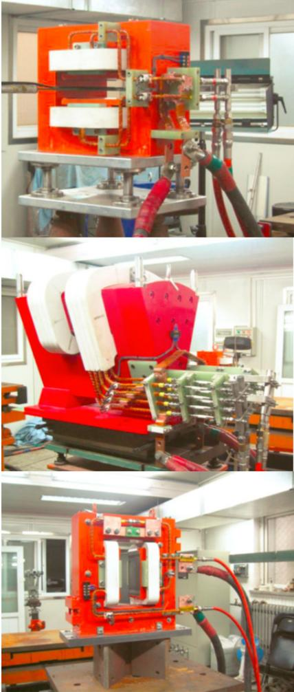
Figure 4: NSC KIPT 100 MeV/100 kW linear accelerator first chicane magnet, 45 degree bending magnet and vertical scanning magnet.
