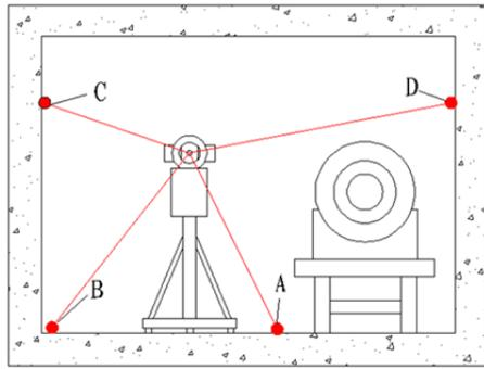
Figure 2: The process of survey target coordinate determinations.
