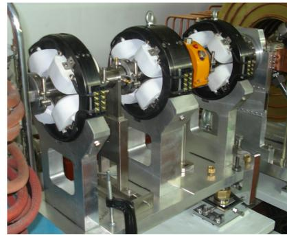
Figure 5: NSC KIPT 100 MeV/100 kW linear accelerator quadrupole triplet.
