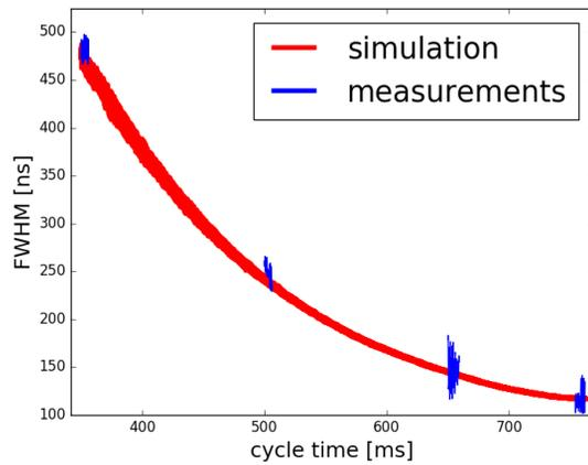
Figure 1: Full-width half-maximum bunch length evolution (50 MeV-1.4 GeV) in simulation and measurements for  $N=5 \times 10^{12}$  ppb.
