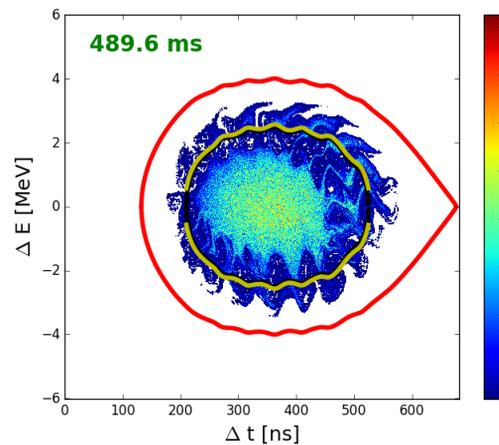
Figure 4: High frequency modulation seen in phase space due to the induced voltage. The separatrix is in red, the yellow curve identifies the trajectory used to compute the emittance measured at 5% of the line density and the color bar indicates the particle density.
