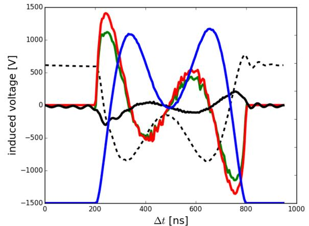
Figure 3: Total induced voltage (green) generated by the bunch described in Fig. 2. The space charge and the closed-loop Finemet contributions are in red and black continuous respectively. The resistive Finemet voltage without reductions (black dashed) is shown for comparison. After saturation of the multi-turn wake, the closed-loop Finemet voltage is capacitive and opposite in sign to space charge. The line density is in blue ( $V_1 = 10$  kV,  $V_2 = 10$  kV).
