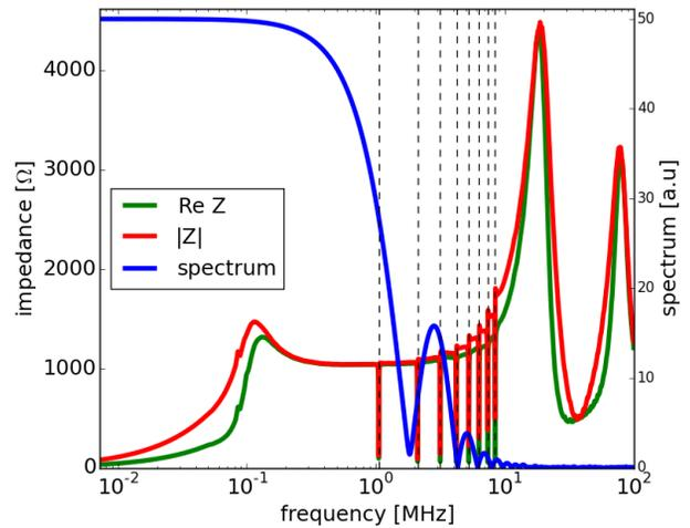
Figure 2: Absolute value and real part of the full PSB impedance model without space charge. The vertical lines indicate the first eight revolution harmonics. The spectrum of a 1 eVs bunch at cycle time 300 ms in bunch lengthening double RF ( $N = 3.6 \times 10^{12}$  ppb) is shown.
