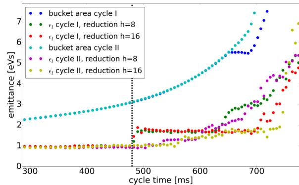
Figure 5: Emittance  $\epsilon_l$  evolution with and without voltage manipulations for high intensity beams using impedance reduction up to harmonic 8 and 16. Instability after 480 ms causes uncontrolled emittance blow-up.
