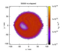
Figure 3: Simulated electron density distribution in a Gabor lens by injecting an electron beam tranversally.
