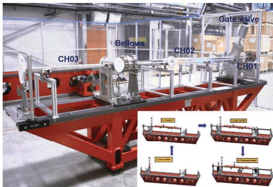
Figure 22: Vacuum assembly on dedicated girder.
