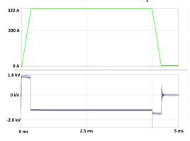
Figure 4: Important features of the simulation results are the 370 µs rise and fall times in the current (top) and that the largest potential to ground anywhere in the system is only 1.62 kV (bottom).
