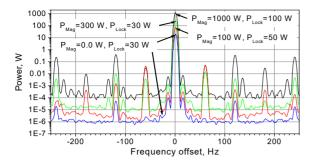
Figure 5: Offset of the carrier frequency at various powers of the magnetron,  $P_{Mae}$ , and the locking signal,  $P_{Lock}$ , [6].
