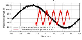
Figure 7: Modulation of the magnetron power managing the magnetron current by a harmonic signal controlling the SM445G HV switching power supply, [6].
