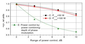
Figure 6: Relative magnetron efficiency vs. range of power variations at various methods of control. Traces C and D are average efficiency of the 1.2 kW magnetron, at the extended current control, [6]. Trace E is the average efficiency of 1 kW magnetrons at power combining, [4], or at management of the depth of phase modulation, [5].
