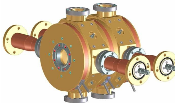
Figure 2: Two-cell, 1.3 GHz buncher cavity CAD model.
