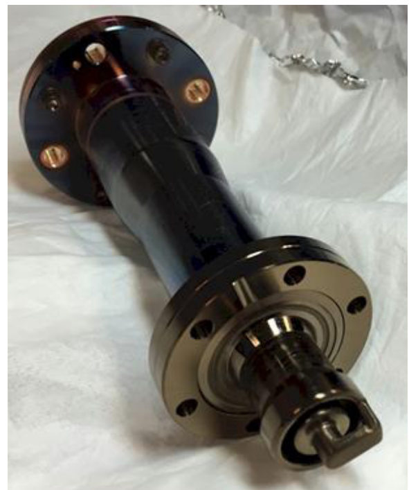
Figure 9: Photo of a coupler assembly after TiN coating.
