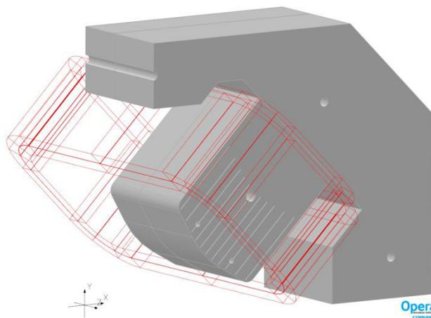
Figure 1: Geometry of 1/8<sup>th</sup> of the yoke.
