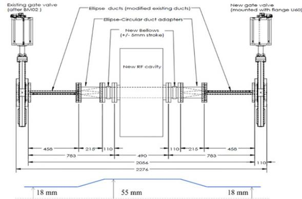
Figure 3: Detailed schematic layout of the new RF cavity.
