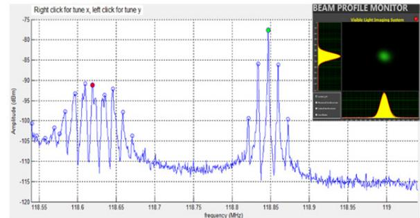
Figure 5: The stable beam and betatron tune spectrums.
