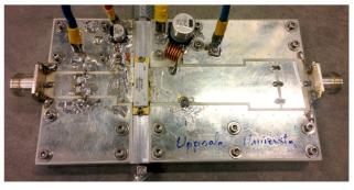
Figure 2: Kilowatt-level power amplifier in a single-ended architecture at 352 MHz.
