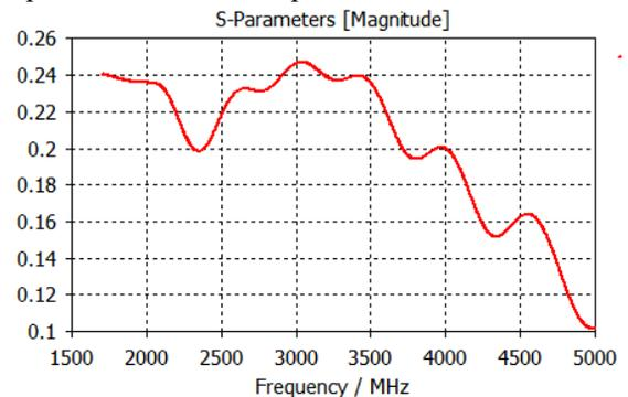
Figure 4: Reflection coefficient of the optimized damper.
