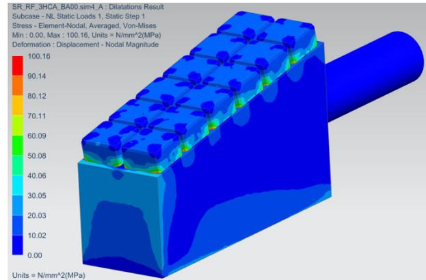
Figure 7. Absorber wedge Von Misses Stresses
