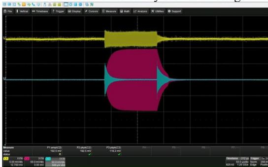
Figure 6: Amplifier and Cavity Voltage Waveforms.
