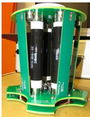
Figure 2: Combiner Balance Resistors with Shielding.
