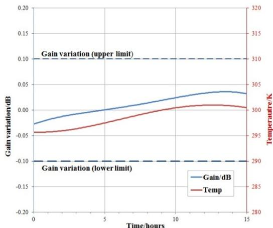
Figure 7: Gain and Ambient Temperature over Time.
