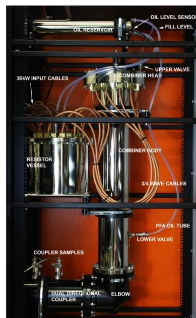
Figure 4: 340 kW Output Combiner.
