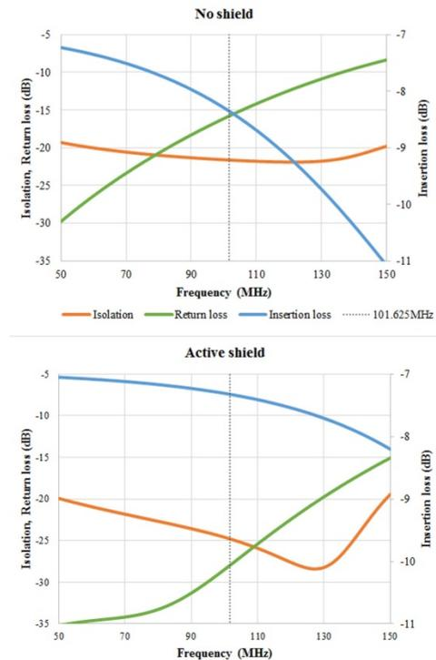
Figure 3: Return Loss and Insertion Loss of Final Output Combiner using Shielded and Unshielded Resistors.
