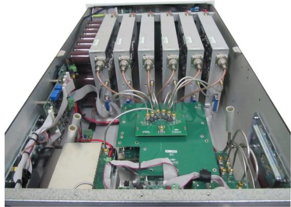
Figure 1: Internal View of 36 kW Amplifier Unit.
