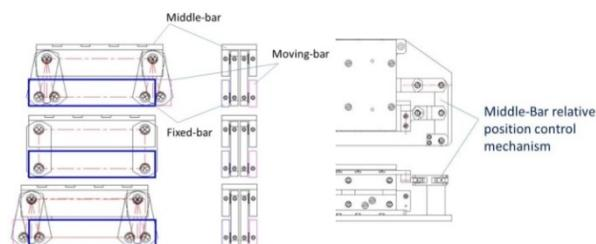
Figure 1: Left: Schematic of the basic parallel mechanism for the flexural-pivots-based linear flexure stage. Right: Schematic of the top-view and a side-view of the middle-bar relative position control mechanism.
