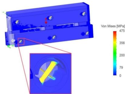
Figure 3: A 3D model shows a FEA study of a single set of flexural-pivots-based linear guiding mechanism with near 6-mm displacement.
