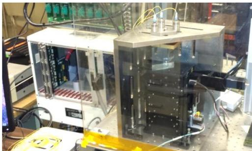
Figure 7: Photograph of the test setup for the T8-55 and T8-56 stages with laser interferometers mounted on an Invar reference frame.
