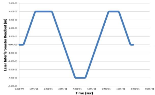
Figure 9: A  $\sim 0.5$  mm/sec driving speed test of the T8-55 vertical flexure stage driven by micro-steps (2 nm/microstep) under a pulse rate of 250k pulse/sec.
