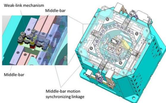
Figure 4: A 3-D model of the special weak-link mechanism applied to the middle-bar motion synchronizing linkage to compensate the transversal relative motions between the middle-bars.
