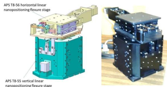
Figure 6: Left: A 3-D model of the combination of the APS T8-55 and T8-56 linear nanopositioning flexure stages for a 2D sample scanning stage system for x-ray microscope. Right: Photograph of the T8-55 and T8-56 vertical and horizontal linear flexural system.
