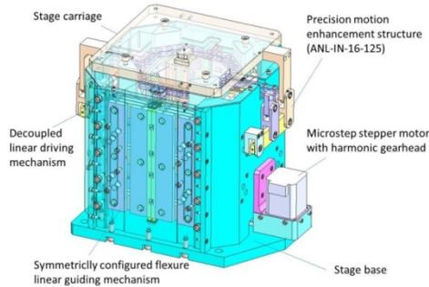
Figure 2: A 3-D model of the APS T8-55 vertical linear nanopositioning flexure stage with symmetric flexural-pivots-based precision linear motion guiding structure and precision motion enhancement structures.
