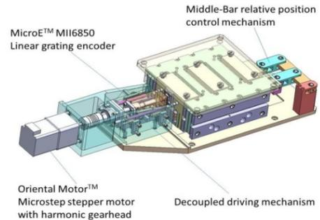
Figure 5: A 3-D model of the APS T8-56 horizontal linear nanopositioning flexure stage.
