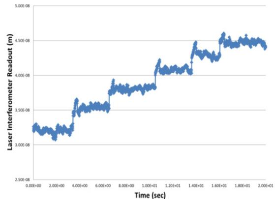
Figure 8: Test for the T8-55 vertical flexure stage positioning sensitivity with five  $\sim 2.5$  nm steps under a microstep stepper motor open-loop control.
