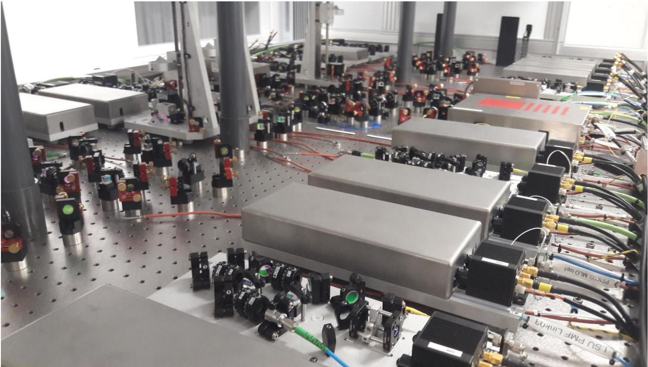
Figure 3: Main optical table for the optical reference generation and distribution. This table currently holds one MLO (the second, redundant MLO is in repair), 3 of 7 optical delay lines, 22 of 24 Link Stabilization units, 74 polarizing beam cubes and more than 250 kinematic mounts.
