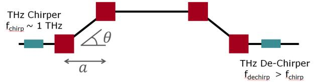
Figure 1: Schematic of a 4 dipole chicane with THz chirping and dechirping.
