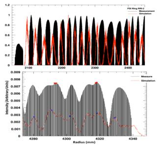
Figure 5: Top: The first few turns, as seen by RRI2, of the modelled beam (red) and the measured beam (black). They are not well matched (exclude first black peak), but reasonably close. Only first 6 are not seen by RRL, and could be better aligned with optimized trim coils. Bottom: The last 7 turns overlapped as seen by RRE4. There is good agreement in the location of the orbits. The magnitude is in arbitrary units for the measured and modelled data.
