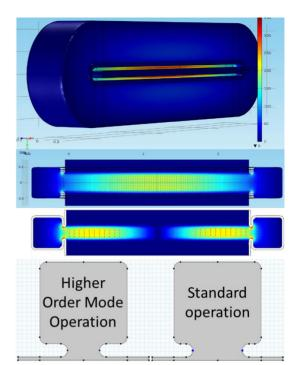
Figure 6: (Top) Rounded ends of a Flat Top Design. (Middle) The electric field of the flat topping mode of the rounded cavity compared to the HOM operational mode. (Bottom) The geometry change required to switch modes in the cavity, which require 4cm of slide in the irises.
