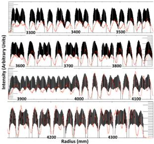
Figure 4: The last 89 turns, as seen from the RRL probe, of the modelled beam (red) and the measured beam (black) are overlapped. There is excellent agreement and all orbits accounted for in the RRL probe.
