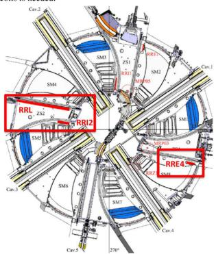
Figure 3: Diagram of the PSI Ring Cyclotron. The location of the three probes used for orbit matching are indicated by thick red lines inside the boxes. Other probes and components are also labelled.
