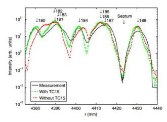
Figure 1: Bi's simulation [7] overlapped with experimental measurements for the last 9 orbits of the Ring cyclotron.
