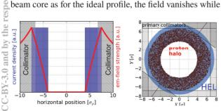
Figure 3: Sketch of the kick from a uniform hollow e-beam distribution (left) and halo input distribution with overlaying HEL beam and collimator positions as used in the HL-LHC simulations (right).
