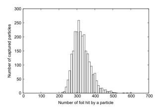
Figure 7: Histogram of number of foil hitting by a captured particle.
