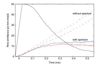
Figure 5: Horizontal (red) and vertical (blue) emittance growth caused by foil scattering. Number of survived particles is plotted in black (full-span=100%). Dashed lines shows the case with infinitely large foil.
