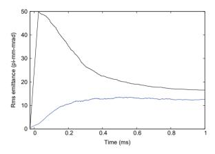
Figure 6: Vertical emittance growth (blue) and number of survived particles (black, full-span = 100%).
