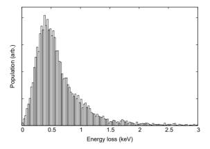
Figure 2: Energy loss at a passage of carbon foil (simulated with GEANT4).
