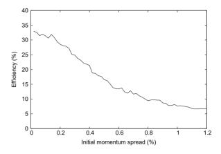
Figure 8: Capture efficiency depending on initial momentum spread.
