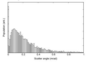
Figure 3: Scattering angle at a passage of carbon foil (simulated with GEANT4).
