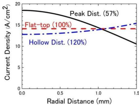
Figure 2: Radial distribution of current density profiles.
