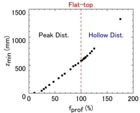
Figure 4: Correlation between the position of emittance minimum and the initial current profile modulation factor  $f_{prof}$ .
