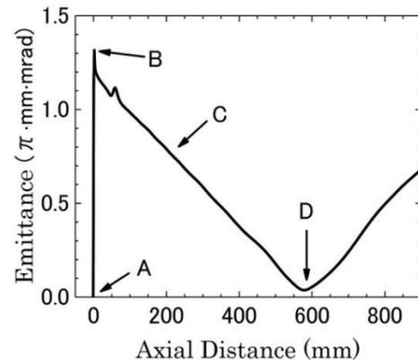
Figure 1: Calculated emittance evolution for the SCSS thermionic gun. The point A, B, C and D correspond to the cathode surface, the emittance maximum, the emittance decreasing point and the emittance minimum.
