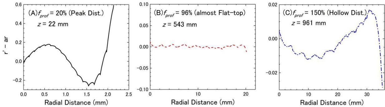
Figure 6:  $r' - ar$  plot at the emittance minimum as a function of the radial distance. Electron beam with (A) Result of peak initial distribution at the axial distance of 22 mm. (B) Result of almost flat-top initial distribution at the axial distance of 543 mm. (C) Result of hollow initial distribution at the axial distance of 961 mm.
