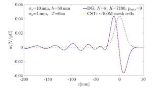
Figure 2: Wake function  $w_s(z)$  for the test tapered chamber with a comparison result from CST Particle Studio<sup>TM</sup> with the direct wake solver. The thin dashed line shows the bunch profile  $\lambda(z)$  scaled to  $w_s(z)$ .
