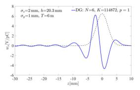
Figure 3: Wake function  $w_s(z)$  shown using only the p = 1 mode for the DESY BC0 vacuum chamber. The thin dashed line shows the bunch profile  $\lambda(z)$  scaled to  $w_s(z)$ .
