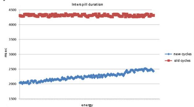
Figure 3 : Comparison between the interspill of the old and the new cycles versus the different carbon energies.
