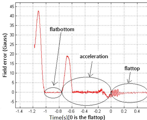
Figure 2 : Magnetic field error from the beginning of the cycle to the extraction under the influence of the B-Train feedback.
