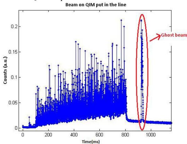
Figure 4: Beam on QIM put in the line for the 400 MeV/u carbon beam.
