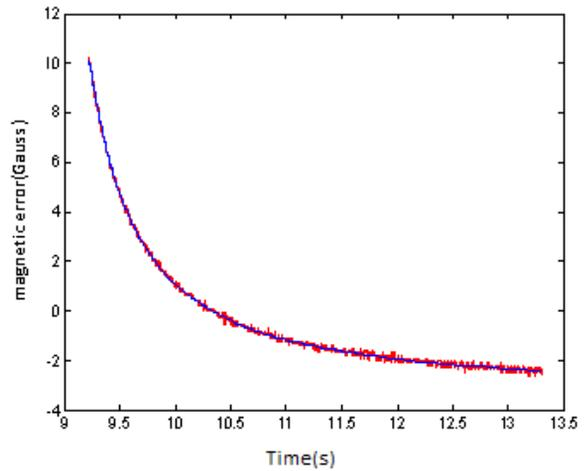
Figure 1: Trend of the magnetic field error after the dipole has reached the current to accelerate 400 MeV/u carbon beams without B-Train feedback.
