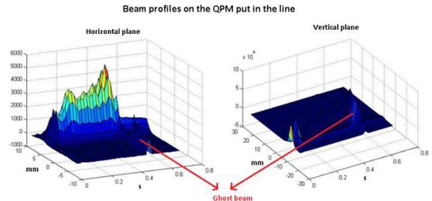
Figure 5: Horizontal and vertical profiles of the 400 MeV/u carbon beam measured by the QPM put in the line.
