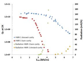
Figure 6: Q<sub>0</sub> vs. E<sub>acc</sub> curves of the bare and dressed HWR-1 at 2K, as well as the radiation levels during the tests.
