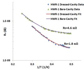
Figure 5: R<sub>s</sub> vs. 1/T curves of the bare and dressed HWR-1 cavity during cooldown from 4.2K to 2K.
