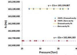
Figure 7: Frequency vs. LHe Pressure when the bare cavity was cooled from 4.2K to 2K.
