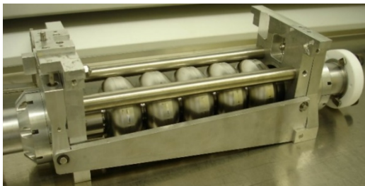
Figure 1: Photo of the capture section of the S-DALINAC injector (the 5 cell SRF \beta=1 cavity in the tuner frame).
