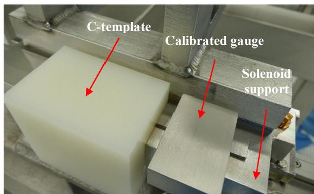
Figure 4: solenoid positioning with a C-template and a gauge
