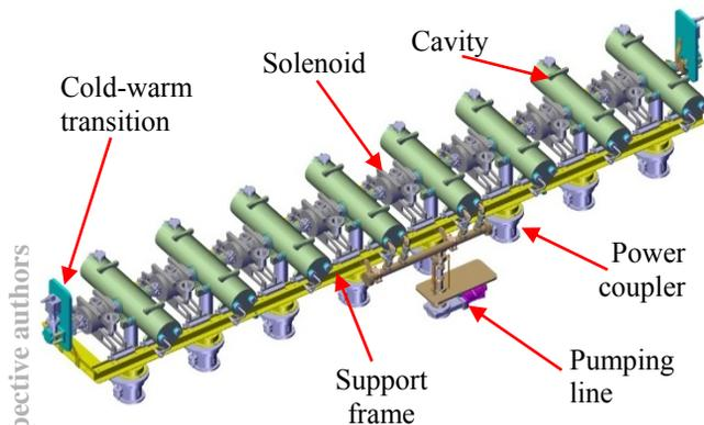
Figure 1: IFMIF cavity string assembly
