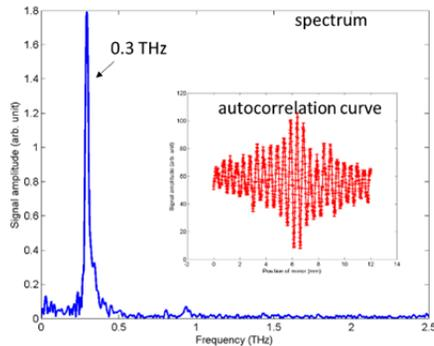
Figure 5: The autocorrelation curve from the interferometer and the spectrum of the 300 GHz DLW.
