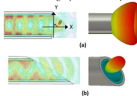
Figure 1: The electric field and the far-field distribution of  $\text{TM}_{01}$  mode at the end of the DLW without angle cut, and as well as the ones in the DLW with an angle cut.
