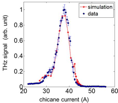
Figure 3: THz energy varies as the chicane current.
