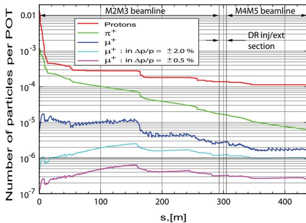
Figure 2: Number of particles per POT along the M2M3 beamline, injection/extraction straight section of DR and M4M5 beamline, showing protons (red line), pions (green line), muons (blue line). Muons with momentum in the range of  $\pm 2\%$  and  $\pm 0.5\%$  with respect to 3.094 GeV/c are shown by light blue and magenta lines, respectively.
