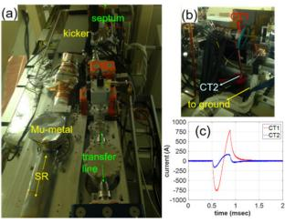
Figure 3: (a), (b) photos of the injection section and (c) eddy current measurements in the real machine.
