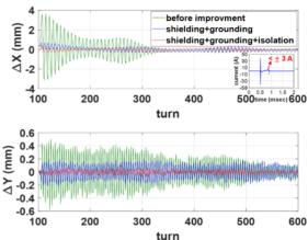
Figure 5: Turn-by-turn BPM data with best matched kicker show betatron oscillations before improvement (green), after mu-metal shielding and grounding with copper cables (blue) and after isolation of current loops (red). The figure insert shows the eddy current after improvements.
