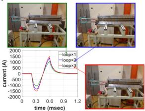
Figure 4: eddy current simulation for different numbers of parallel current loops.
