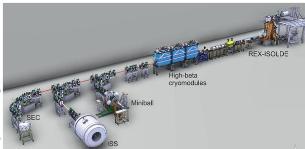
Figure 1: A 3D visual of the HIE-ISOLDE linac, composed of three cryomodules, and the three experimental stations in the HEBT. At the end of the first beam line, XT01, Miniball is located, at the second, XT02, the ISOL Solenoidal Spectrometer, ISS, and the third, XT03, is reserved for movable setups. In the drawing, XT03 is occupied by the scattering chamber, SEC, which is presently connected to XT02. [1]
