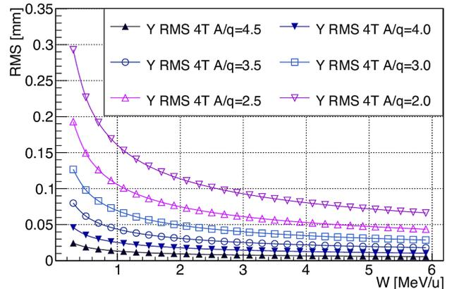
Figure 5: Energy dependent Y RMS measured on BPMs after correction for the ISS magnetic stray field at  $A/q = 4.5$  and various scaling of  $A/q$ .
