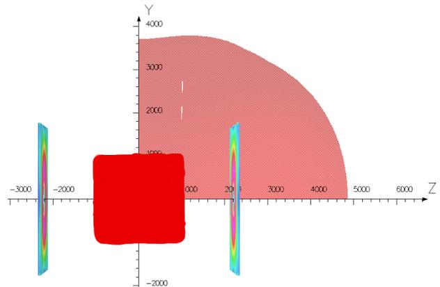
Figure 2: 3D simulations of the solenoid's magnetic field with the latest magnetic shielding design. In addition, the envelope of the 5 G limit around the ISS magnet is shown in light red.
