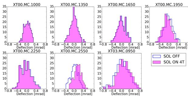
Figure 6: Corrector settings along XT00 and XT03 for  $\sigma_y = 0.1 \text{ mm}$  misalignment of the quadrupoles with and without the presence of the ISS magnetic stray field for a beam energy of  $0.3 \text{ MeV/u}$ .
