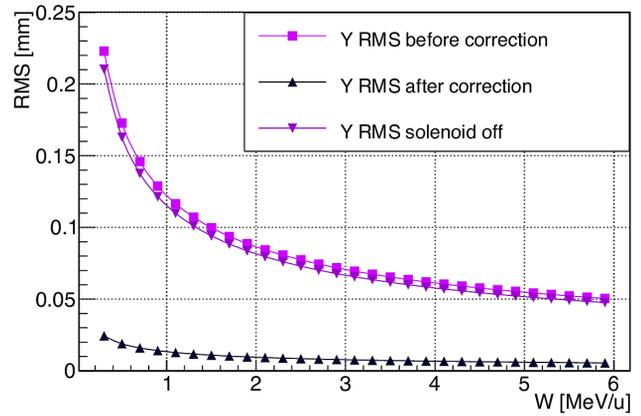
Figure 4: Energy dependent Y RMS measured on BPMs before and after correction as well as after turning the ISS magnet off.
