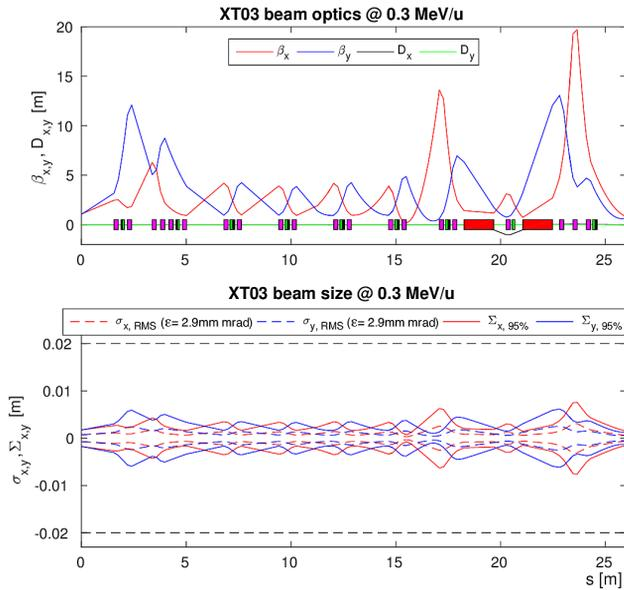
Figure 3: Optics and beam sizes along XT03.
