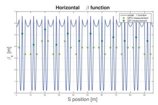
Figure 2: Horizontal  $\beta$  function measured in SQFO and SQFI magnets locations.
