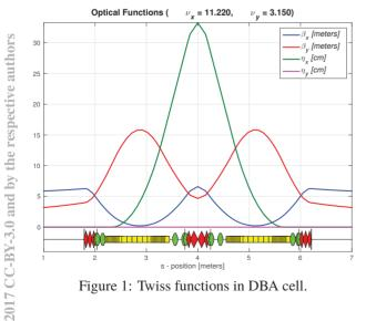
Figure 1: Twiss functions in DBA cell.
