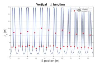
Figure 5: Vertical  $\beta$  function measured in HCM and VCM corrector magnets locations.
