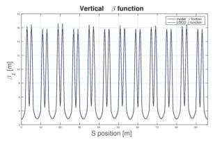
Figure 7: Vertical  $\beta$  function obtained using LOCO algorithms.
