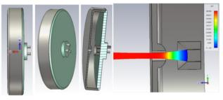
Figure 3: Designed spherical cathode electron gun and particle trajectory.
