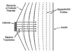
Figure 2: Schematic of the flat cathode pierce electron gun.
