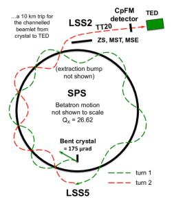
Figure 1: Schematic of the crystal-assisted extraction scheme.
