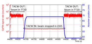
Figure 4: TT20 CpFM signal rate (red) vs. TACW position (blue) [19].
