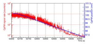
Figure 6: TT20 CpFM signal (red) and position (blue) vs. time as it is moved out of the extracted beam [19].
