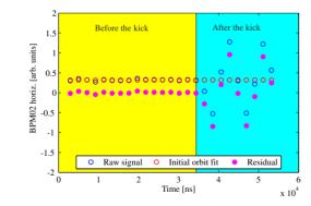
Figure 2: The BPM reading in time before and after the kick.
