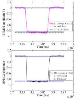
Figure 7: The rise and falling times evaluations.
