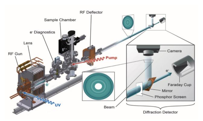
Figure 2: The layout of the initial operational configuration of the UED apparatus in Building 912 at Brookhaven National Laboratory.
