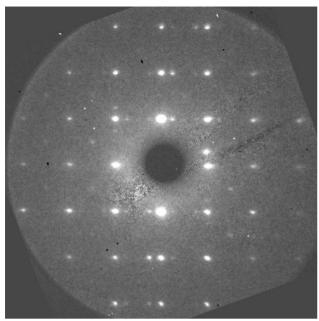
Figure 3: Present operational diffraction pattern (March 2017). Supersctructure spots can be observed around main peaks.
