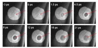
Figure 4: Electron beam image of the copper grid profile with imposed laser pump spot in it at different time.
