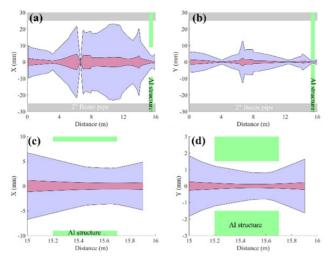
Figure 3: Horizontal (a) and vertical beam (b) envelope along the double EEX beamline. The red envelopes show the sigma for x and y, and the blue envelopes shows the full size of the beam for x and y. (c) and (d) shows the beam envelopes near the structure.
