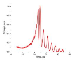
Figure 4: Charge time delay scan using the Channeltron.
