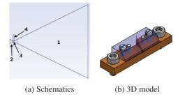
Figure 1: Schematics and 3D model of the Horn gun. Left figure numbers indicate: 1 - big horn for THz pulse coupling, 2 - small horn for THz reflection, 3 - accelerating waveguide, 4 - slit. Upper side on the right figure is made transparent for details.
