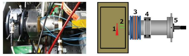
Figure 6: Experimental setup including the Horn gun (1), parallel plates (2) air coil (3), PCB steerer (4) and MCP (5).
