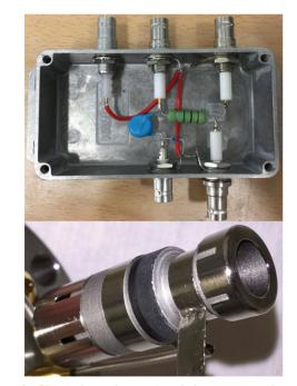
Figure 3: Channeltron (bottom) and electric circuit box (top).
