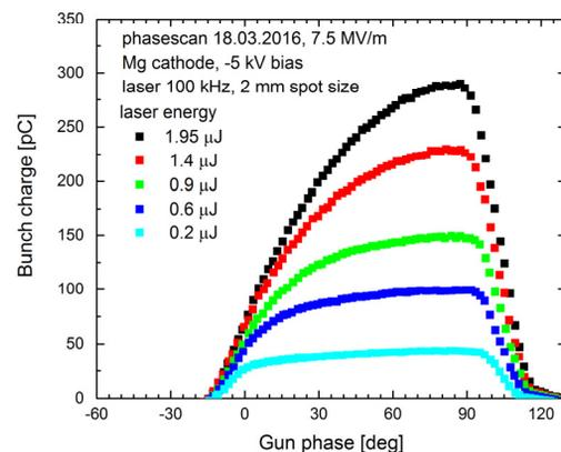
Figure 2: Bunch charge as the function of SRF gun phase.
