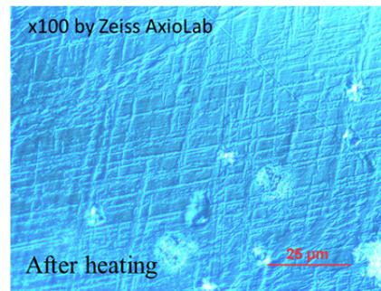
Figure 7: the topography of mono-crystal Mg sample soon after heat treatment (already exposed in air).
