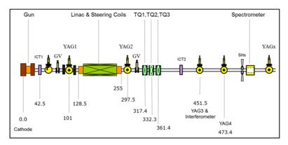
Figure 1: The AWA witness beam-line showing various elements and distances from the photocathode in units of mm.
