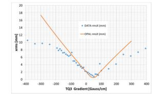
Figure 2: Horizontal RMS beam size vs. magnetic focusing strength; Q=1.3nC. Figure 2 shows an OPAL-t (hereafter 'OPAL') simulation of the horizontal RMS beam size in orange compared with measurements.
