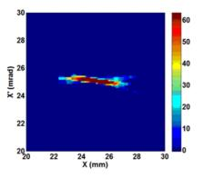
Figure 6: Trace space (x, x') reconstruction using OPAL simulated beam images generated at YAG4.
