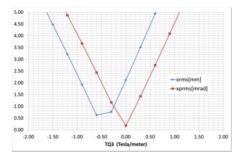
Figure 4: Horizontal RMS beam size and divergence vs. TQ3 quadrupole strength.
