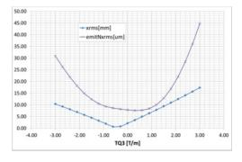
Figure 3: Horizontal (x) RMS beam size and x emittance vs. TQ3 gradient for beam with Q = 1.3 nC.
