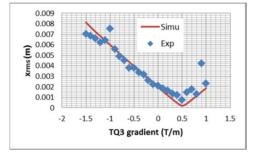
Figure 5: Horizontal RMS beam size vs. quadrupole (TQ3) gradient (Tesla/meter).
