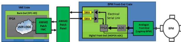
Figure 5: Button BPMs signal acquisition and processing scheme.
