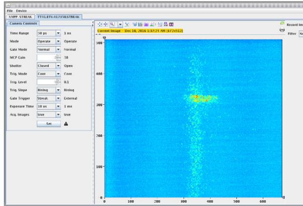
Figure 4: Streak camera image of the proton bunch and laser pulse taken during the December 2016 physics run.
