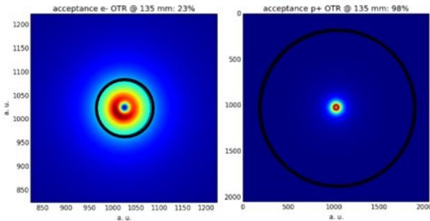
Figure 2: Simulation of OTR light collection from the electron beam (left) and the proton beam (right). Signal falling outside the black circle is not collected by the optical system (the images have a different spatial scale).
