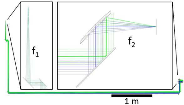
Figure 3: Simulated layout of the streak camera line. The insets show the off-axis parabolic mirrors at the source ( $f_1$ ) and image ( $f_2$ ) side. On axis illumination (Blue) and off-axis illumination (Green).
