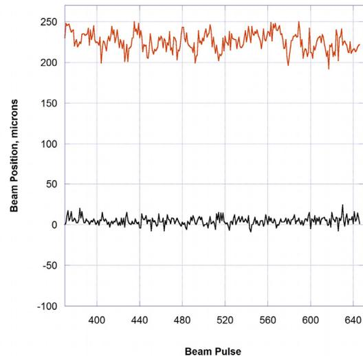
Figure 6: Horizontal (black) and vertical (red) beam position evolution of a 150 pC electron bunch as measured in CTF3.
