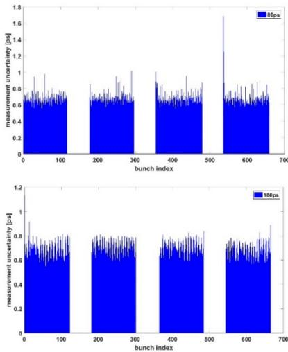
Figure 6: Resolution of bunch phase measurement of 80ps interval (up) and 180ps interval (down).
