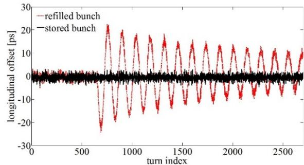
Figure 9: Longitudinal offset of the injected bunch separated from the stored one.
