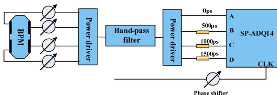
Figure 7: Hardware block diagram of  $90^\circ$  phase difference measurement system.
