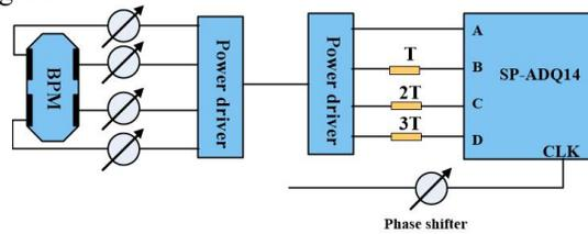
Figure 5: Hardware block diagram of the bunch-by-bunch phase measurement system.
