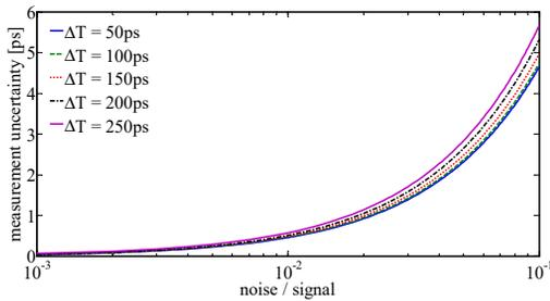
Figure 2: Phase measurement uncertainty simulation of the zero-crossing detection method.
