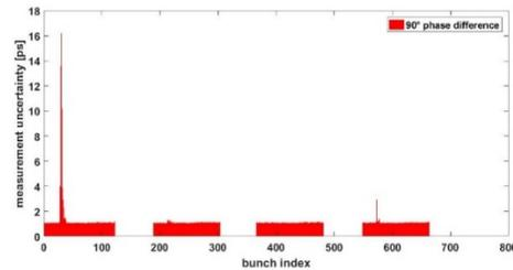
Figure 8: Resolution of bunch phase measurement of  $90^\circ$  phase difference.
