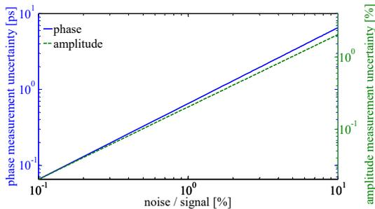
Figure 3: Phase and amplitude measurement uncertainty simulation of the IQ sampling method.
