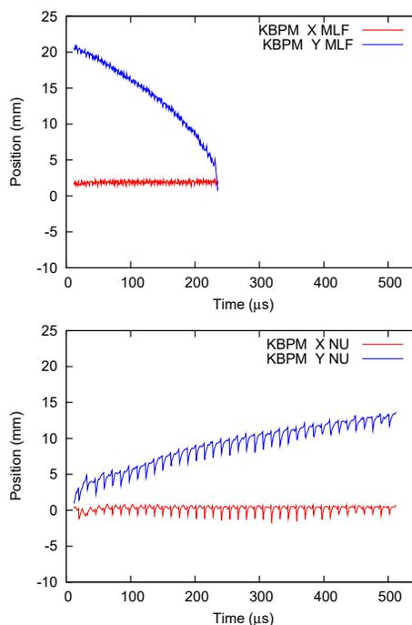
Figure 1: Plots of beam position vs. time for K-BPM. Positions for both the MLF and the NU modes are shown.
