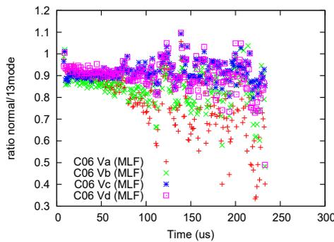
Figure 3: Cell 6, 7 BPM324 voltage amplitude ratio between normal operation and 1/3 mode for the MLF beam.
