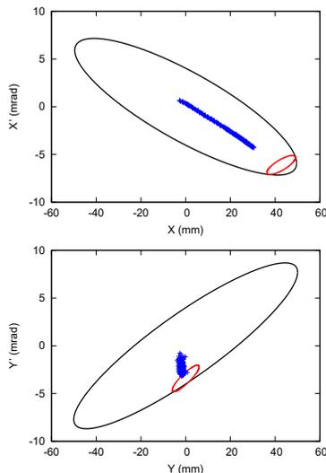
Figure 4: The reconstructed injection beam position in phase space for the 1/3 mode.
