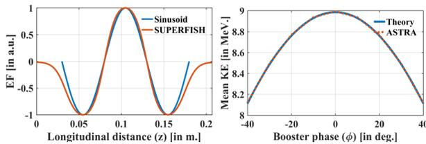
Figure 1: Left: Comparison of theoretical & ‘realistic’ (simulated with SUPERFISH) electric fields inside the booster. Right: Mean kinetic energy obtained from ASTRA and the theoretical model (Eq. (1) + 5.25 MeV) with booster phase ( $\phi$ ).
