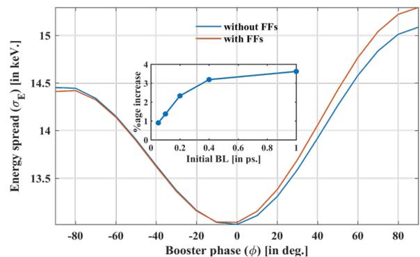
Figure 3: Bunch energy spread with booster phase, with and without the fringe fields for an initial bunch length of 100 fs at the entrance of the booster. FFs: fringe fields.
