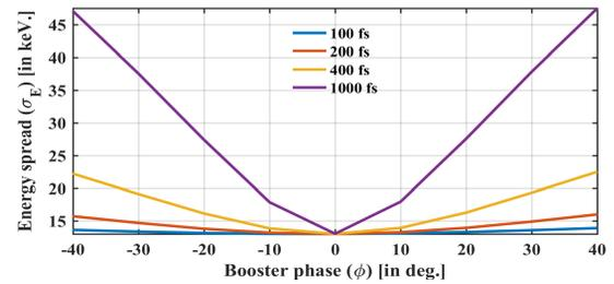
Figure 2: Bunch energy spread with booster phase, without considering space charges and fringe fields.
