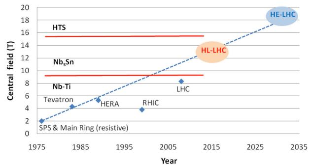
Figure 3: Dipole fields for hadron colliders as function of time (courtesy L. Rossi).
