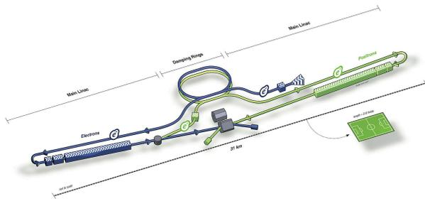
Figure 6: Schematic layout of the international Linear Collider (ILC).
