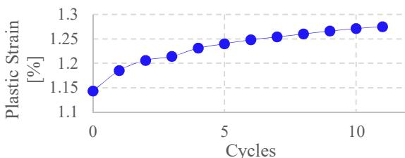
Figure 4: Plastic deformation after load-unload cycles in 11T azimuthal cables.
