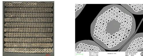
Figure 1: Cross section and micrography of a Nb<sub>3</sub>Sn Cable.
