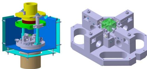
Figure 2: Test rig inside the cryostat and measuring sled.
