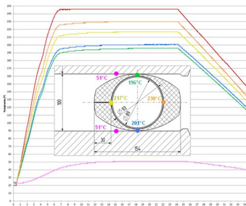
Figure 7: Temperature distribution in the dipole cross section.
