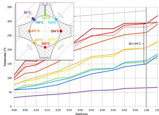
Figure 8: Temperature distribution in the quadrupole cross section.
