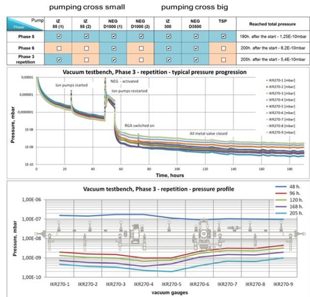
Figure 4: Vacuum test bench pressure progression and profile Phase 3.
