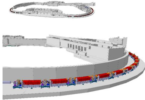
Figure 1: Layout of HESR (High Energy Storage Ring).
