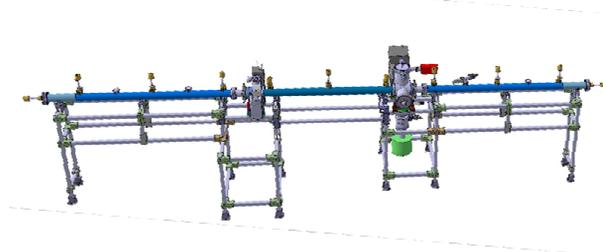
Figure 2: Layout of the vacuum test bench.
