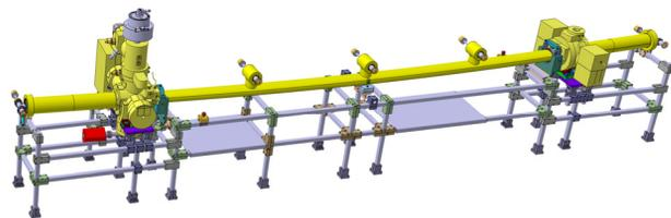
Figure 3: Layout of the bakeout test bench.
