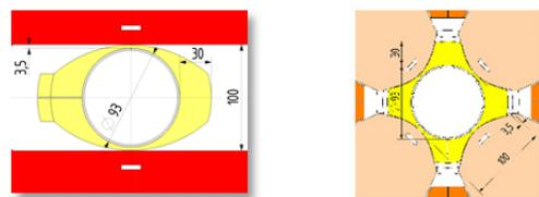
Figure 5: Limited space inside the dipoles and quadrupoles.
